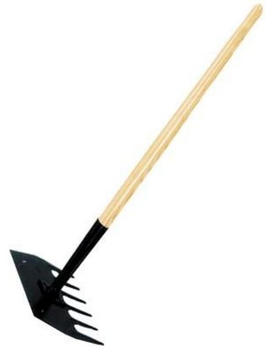
The McLeod helps greatly in shaping the bench/tread after cutting in the back edge. The ‘McLeoder’ is extremely important in keeping everyone in the trail crew focused on the tread design and out slope.
