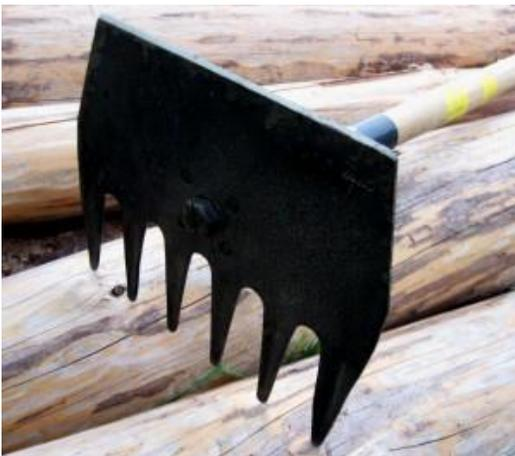
Storing the McLeod is easy. The tines (rake part) should be masked into the ground on the up slope of tread/bench and the handle perpendicular to the tread. Never leave a tool on the tread or construction area.
